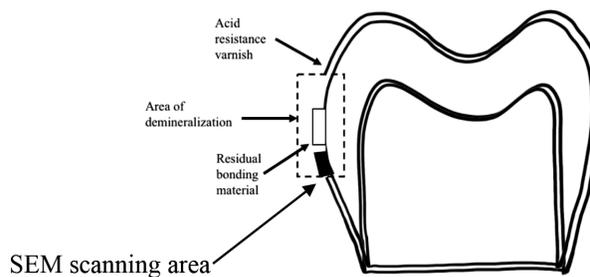
**Fig. 2** Scanning the study area by scanning electron microscope (SEM)
