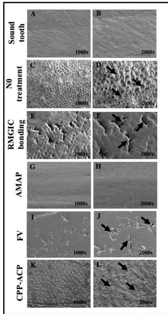
**Fig. 4.** Characterization of surfaces of the enamel specimens by SEM at magnifications of 1000x and 2000x of a sound tooth (Fig. 4A, 4B) after 96 hours of acid exposure in the non-treated group (Fig. 4C, 4D), the RMGIC bonding group (Fig. 4E, 4F), the AMAP group (Fig. 4G, 4H), the FV group (Fig. 4I, 4J), and the CPP-ACP group (Fig. 4K, 4L). The arrows point to porosity caused by demineralization, which occurred over the entire labial surface.
